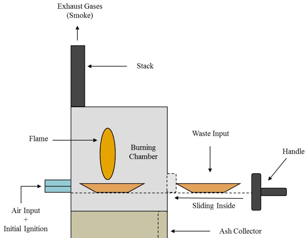
Fig. 6: Schematic diagram of hospital waste incinerator.
