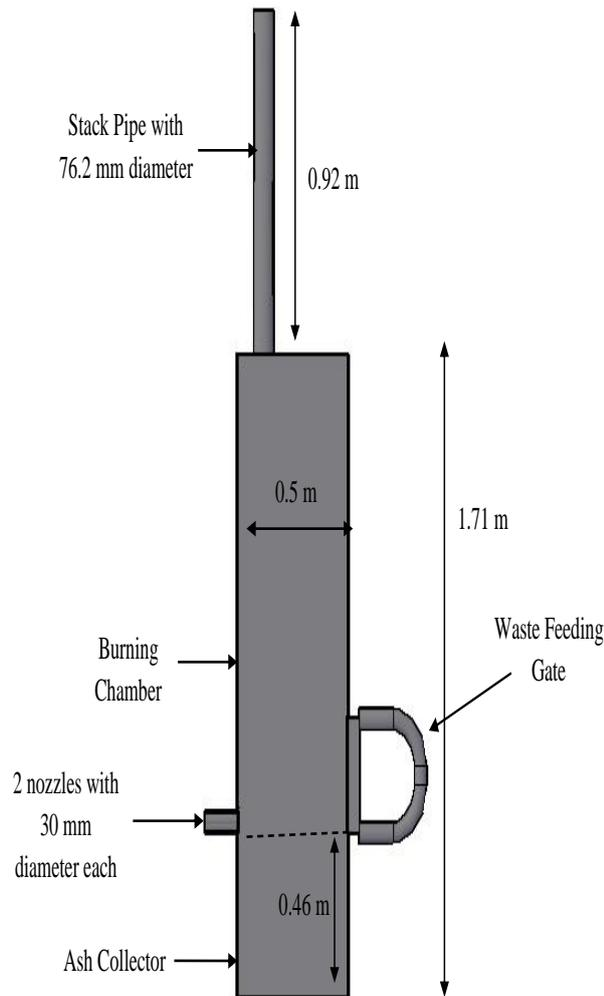
**Fig. 7:** 2-D view and dimensions of designed fixed bed hospital waste incinerator.
