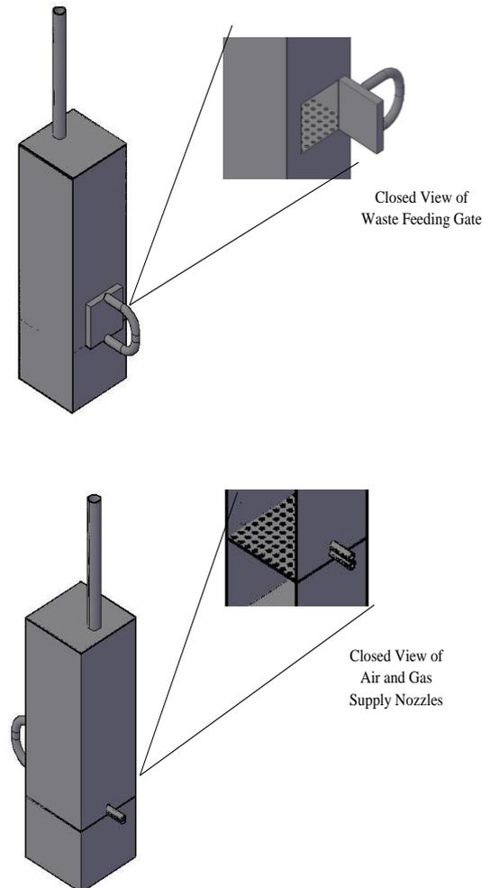
**Fig. 8:** 3-D view of fixed bed hospital waste incinerator.
